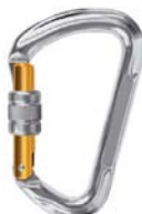
K5330PE VIA FERRATA / lock 30 kN Light alloy carabiner specially designed for via ferrata, rope parks and adven- ture centers ■ quick and easy automatic spring locking ■ big gate opening for clipping on big diameter wires ■ key lock to avoid snagging when clipping and unclipping ⬆ 30 kN ⬆ 8 kN ⬆ 9 kN gate opening (d) 26 mm Weight: 87 g (3.1 oz) CE 0333 ■ EN 12275
